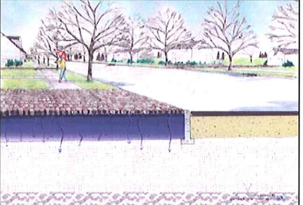
Duration of Storm Event - Storage & filtration/infiltration
